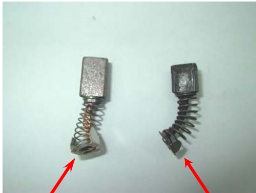
New Motor Brush Worn Motor Brush (Fig 41)
